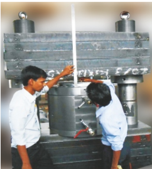
3. Typical View of a Roll Force Cylinders Bore \varnothing 800mm x Piston Rod \varnothing 750mm x Stroke 272.5mm --Fixing of Pressure Pad (Rocker Plate)
