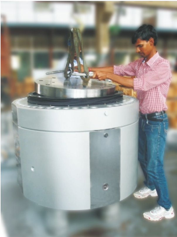
3. Typical View of a Roll Force Cylinders Bore \varnothing 800mm x Piston Rod \varnothing 750mm x Stroke 272.5mm --Fixing of Pressure Pad (Rocker Plate)
